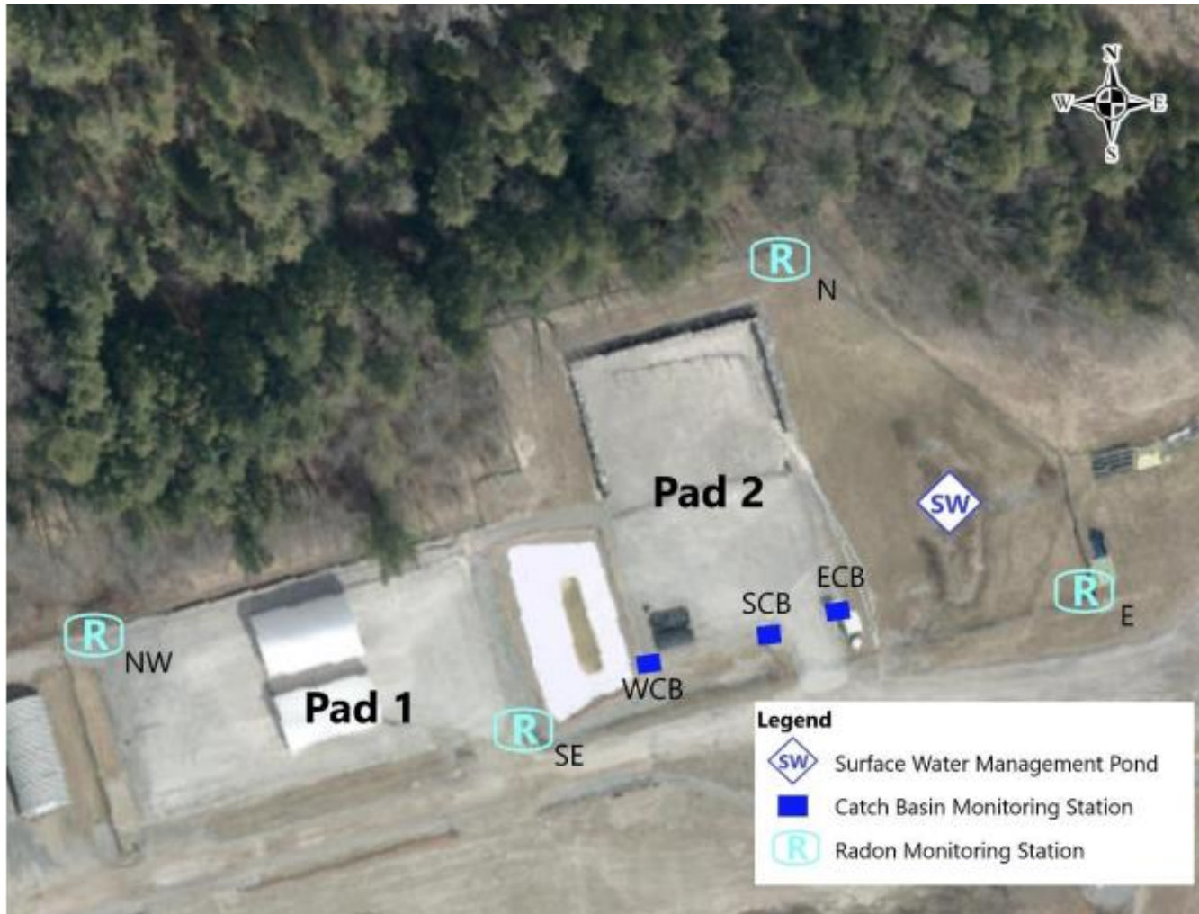
Figure 34: Temporary Storage Site Monitoring - Pine Street Extension Temporary Storage Site
